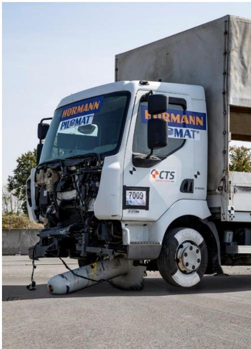
**Image 3:** In the event of a vehicle impact, the OktaBlock from Hörmann tilts forward and the base plate with its prongs wedges between the vehicle and the road surface, quickly bringing the vehicle to a stop.
