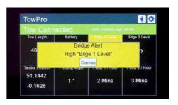
Essential data identified in the Advanced Tow Protection collaboration transmitted live from the tender includes information about how long the bilge pumps have run in the past hour, bilge water levels, battery charge, as well as external factors including continuous measurement of surfing and yawing, trim and pitch, list angle and rolling. All of these are considered key safety indicators of emerging problems with the tow. which can be viewed on TowPro's screen display on the superyacht.
