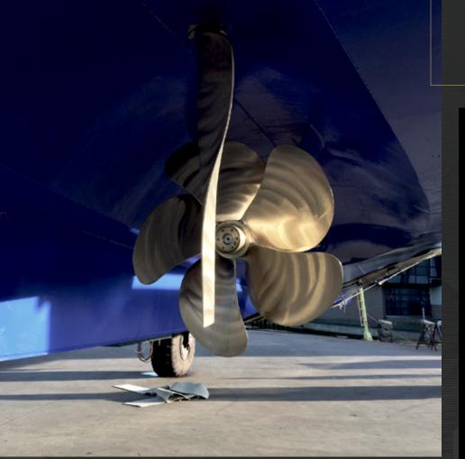
When considered as part of a fully optimised propulsion package, well-designed rudders can have a notable impact on fuel consumption and maximising boat speed, as well as directly reducing noise, vibration and cavitation levels.
