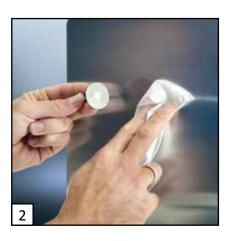
Clean fastener and substrate with scotchbrite and solvent
