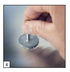
Firmly push the part onto the substrate until the adhesive squeezes out from under the base. Depending on the adhesive selected the fastener is ready for use in 15 - 45 minutes.
