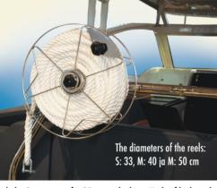
Includes 3 connectors for 25 mm rail tubing. Made of high-grade electro-polished stainless steel. Connectors also available in 22. 30 and 32 mm. The reel can be attached with screws on a flat surface (under hatches, on a panel etc.).
