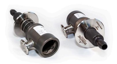
Test tool supplied with a hose to collect water to a container for measuring of flow, k-factor and flushing of pipes.
