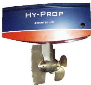
Illustration Hy-Prop 250, manoeuvrable through 2x90 degrees
