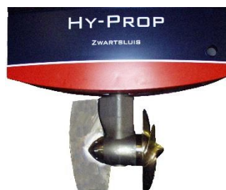
Illustration Hy-Prop 250, manoeuvrable through 2x90 degrees
