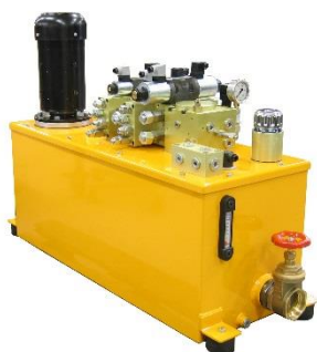
Maritime system, long design 160 litre reservoir equipped with 24 V DC electric motor, suction connection and customer-specific location of sight glass.
