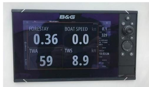
*smarttune sending rig loads to boat instruments*
