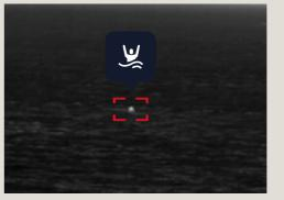
Keep selected object in the screen center, e.g. monitoring a person over board or tracking a tender.
