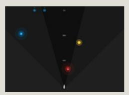
Forward panning. Intelligent alarm alerts of an impending collision risk with objects in the vessel's path.
