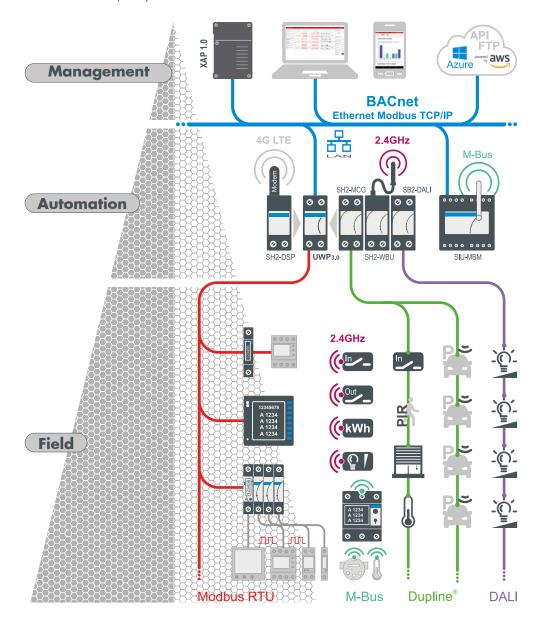
While on one hand UWP 3.0 significantly simplifies the field level of HVAC and lighting wiring without increasing material costs, on the other hand it reduces both commissioning and BACnet integration time.
