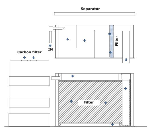
Separator - sedimentation/coarse filter: 1200 x 690 x 498 mm Filter: 1200 x 690 x 800 mm with 300 liter absorber Carbon filter: 600 x 1000 mm (barrel) with 150 liter carbon Max flow: 1,5 m3/h Recommended flow: 1,0 m3/h
