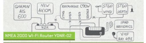
The Router connects all marine and mobile devices easily. It supports all popular marine protocols, is compatible with virtually all marine software, and even allows management of your vessel from a web browser without internet connection or installed software.
