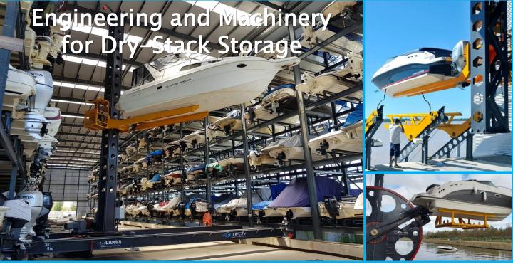
The Gantry System consists of 1 boat stacker crane and 2 launchers per dry-stack for a rapid delivery solution
