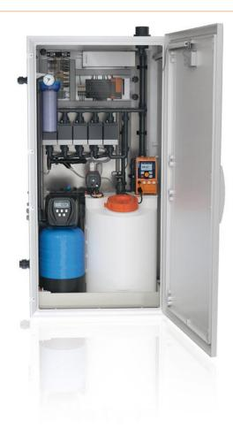
CHLORINSITU® IIa is a compact on-site electrolysis plant for the production of a low chlorate hypochlorite solution from common salt and electrical energy. A particular advantage is the simple process control and high plant safety due to integrated ventilation.
