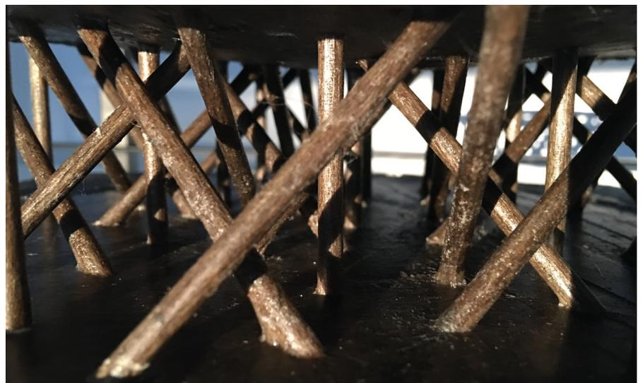
*4mm diameter flax fibers infused with bio-based epoxy Infugreen 810.*
