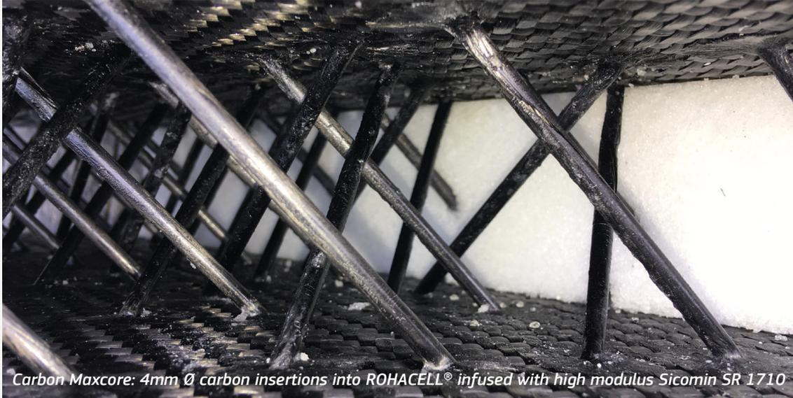
*Carbon Maxcore: 4mm Ø carbon insertions into ROHACELL® infused with high modulus Sicomin SR 1710*
