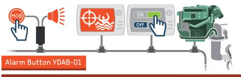
The Alarm Button is a multifunctional NMEA 2000 device with wires for connection of an external button with an LED indicator and a standard 4 or 8 Ohm sound speaker. It contains a 10W audio amplifier inside and a bank with 28 sound signals (car anti-theft alarm, ship horns, whistles, tone signals, etc.).
