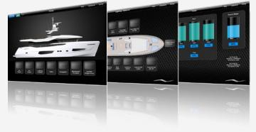
With the introduction of the 26XP series Numarine once again wanted to use the effective, reliable and flexible E-Plex system they had incorporated into other lines. Overall, the 26XP E-Plex system provides control and monitoring from one touchscreen panel and an iPad interface, giving mobile as well
