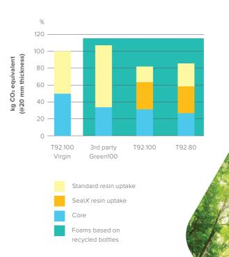
Due to its unparalleled resin uptake, the virgin-PET based **AIREX® T92** version already outperformed the 3<sup>rd</sup> party's PET core materials based on recycled raw material. These sustainable credentials of **T92** are now confirmed and expanded with the renewed, green **AIREX® T92** containing recycled post-consumer bottles.
