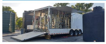
A full systems demonstrator that is a customized design using your preferred off-the-shelf componentry that can process up to 3 tonnes per day. It is also a mobile skid-mounted unit that is small enough to be fitted onto the back of a truck.
