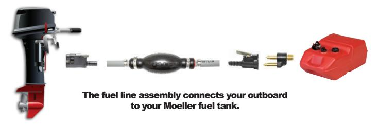
Fuel line assemblies must comply with both USCG safety regulations and EPA evaporative emissions requirements. Hose and primer bulbs are also required to meet low permeation standards. Below deck fuel line assemblies must conform to ABYC H-24, and outboard fuel assemblies must be installed in accordance with ABYC H-25. Hoses which are exposed to sunlight—this includes nearly all hoses used in outboards—must also be UV resistant.
