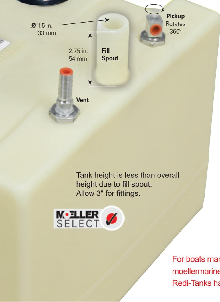
Tank height is less than overall height due to fill spout. Allow 3" for fittings.
