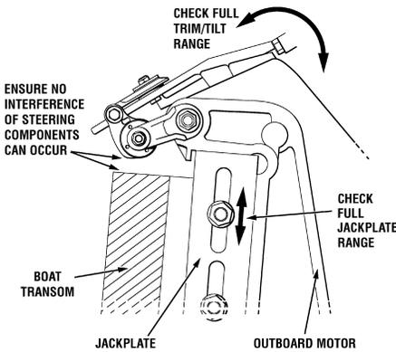
Operational interference of the steering cylinder/cylinder fittings and jackplates/transom/splashwell can occur under certain conditions. Check installation thoroughly throughout the full range of Motor Tilt, Jackplate Height and Trim before making final installation.
