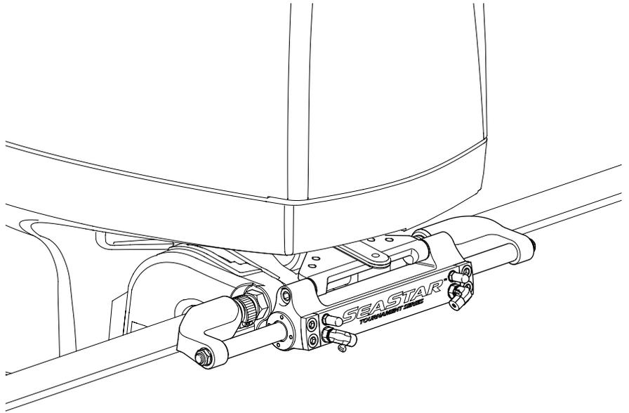
Figure 3-11. Single Engine – Single Cylinder Configuration.
