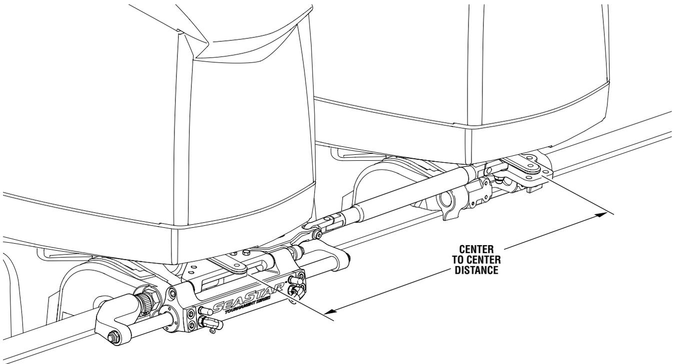
Figure 3-12. Twin Engine – Single Cylinder (Starboard) Configuration.
