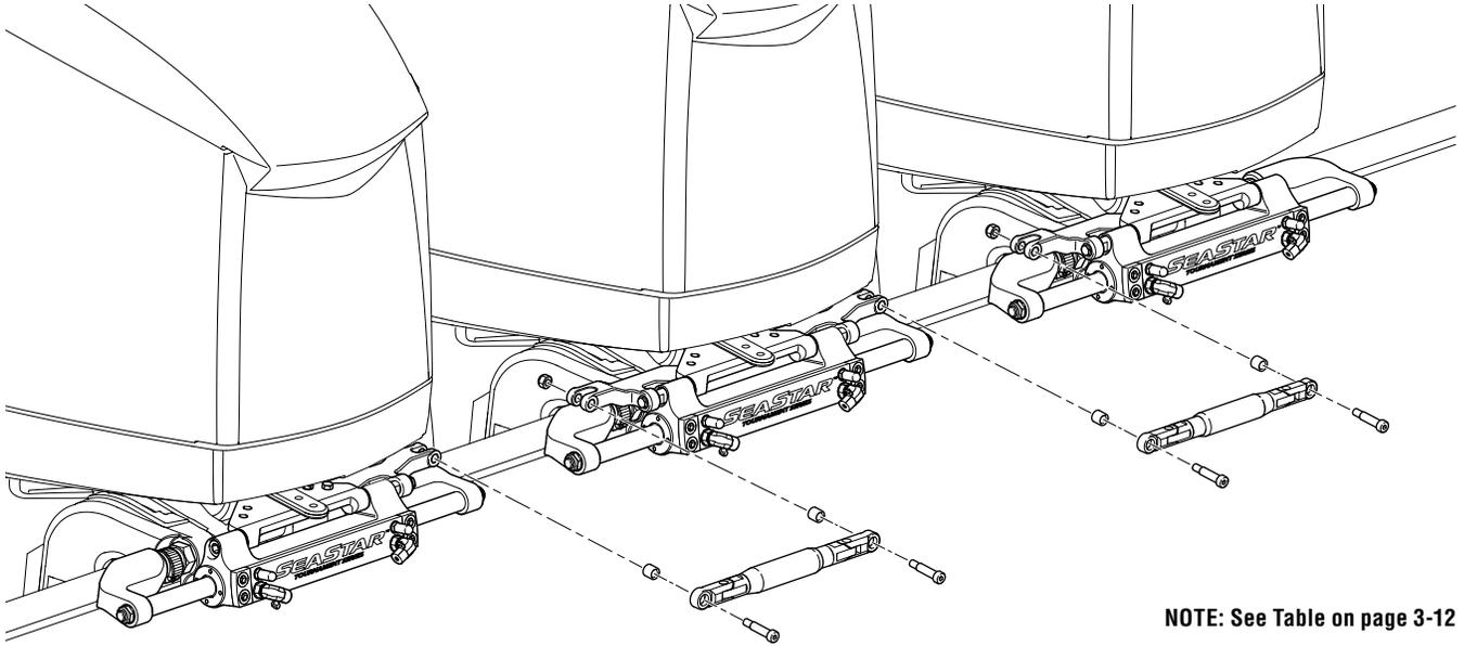
Figure 3-15. Triple Engine – Triple Cylinder Configuration.
