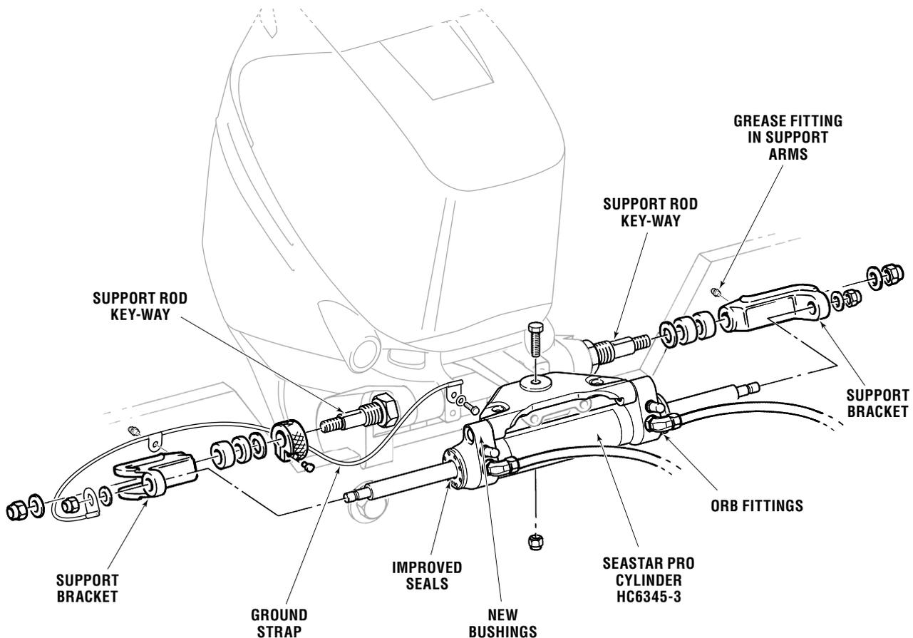
Figure 3-6. Cylinder Part# HC6345-3 shown.
