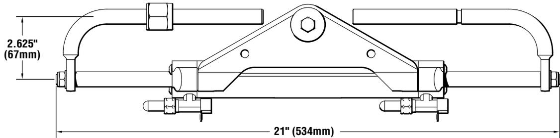
SEAL KIT = HP4600    TEE/BLEEDER KIT = HF4202    SUPPORT ROD/NUT/CLIP = HP6050    PIVOT PLATE SEE page 1-5
