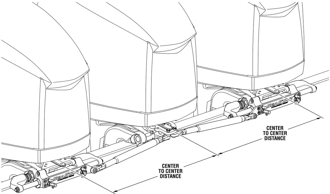
Figure 3-14. Triple Engine – Dual Cylinder Configuration.
