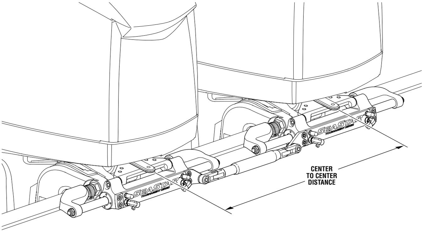
Figure 3-13. Twin Engine – Dual Cylinder Configuration.
