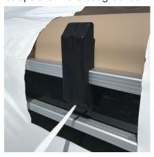
Bring strapping up to the support post and afix to the opposite side strapping with a buckle - strapping should be pulled tight by hand
