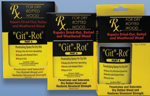
Unique two-part liquid epoxy saturates and restores original strength to wood by **penetrating** the rot. Actually works with the loose rotted fibers. Wood must be dry. Apply by injecting into wood. Will soak into wood by capillary action. One-half hour pot life after mixing. Cures overnight. Sandable and paintable, can be drilled and screwed. Compatible with fiberglass resins, epoxies and most sealants. Great for transoms, stringers and cabin roof rot in both fiberglass and wood boats.
