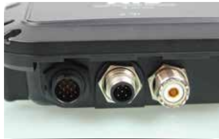
Multiple data interfaces – NMEA0183, NMEA2000, USB
