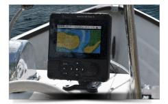
Certifed IPx6 & IPx7 weatherproof. Shock & vibration protection. Suitable for external installations.
