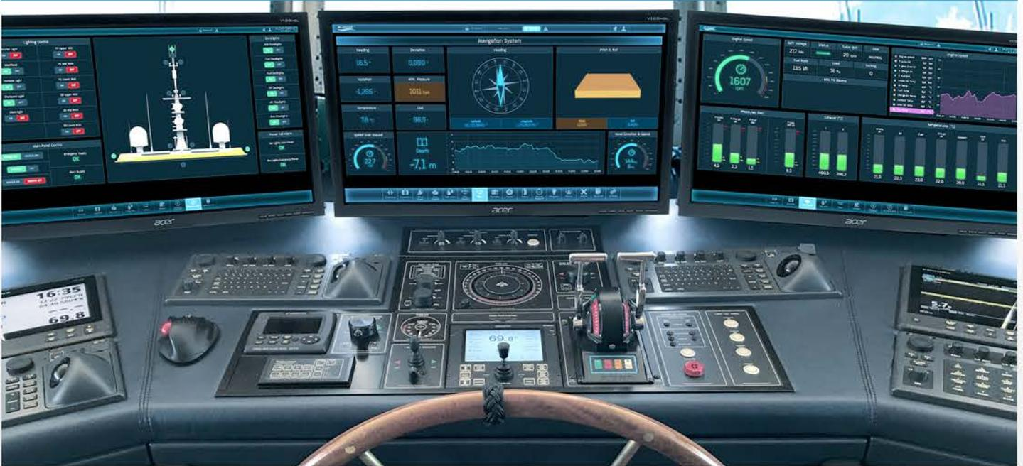
ETY's **BLUEWAVE™** Dashboard and Alarm Monitoring System integrates real time signals on board via cutting edge automation devices.
