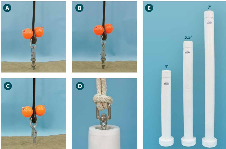
The Hazelett Spar Buoy (E) is a 6-inch diameter polyethylene tube that is filled with foam and concrete for ballast. Wave action does not have as much of an impact on our spar buoy as it does on a ball floating on the surface, so wear on the metal-to-metal connection between shackle and anchor is minimized. Our spar buoy has a pocket molded into the top that houses a stainless steel swivel (D) where bridles or pendants attach, and a removable boot covers the swivel to protect the boat's hull.
