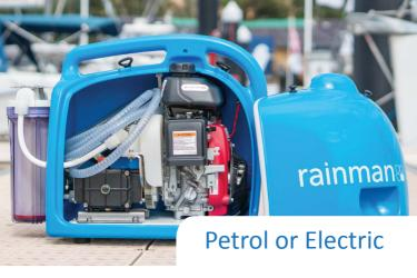
The Rainman Pressure Supply Unit (PSU) is available with a Honda petrol (gasoline) engine, or multiple electric options. Two AC options operate at either 230V/50Hz or 115V/60Hz, and a lower power 12VDC version.
