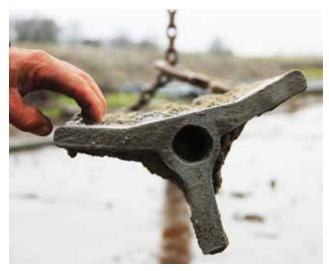
The LDE (fin) element transfers the shear force to the soil.
