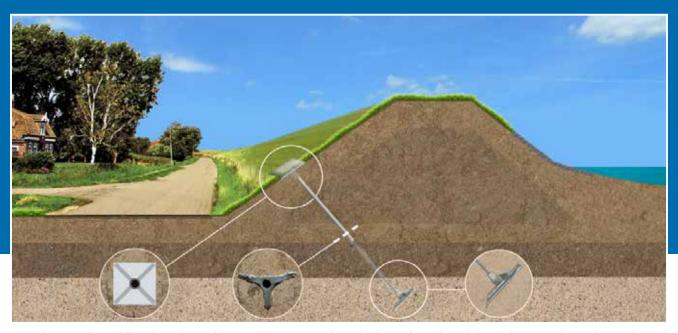
The JLD-Dike Stabilizer is made up of four components: LDP (cap plate), LDE (star-shaped element), JLD-Anchor and an anchor rod.
