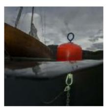
Only the lower swivel (under water) shall be used for mooring. Do not expose the buoy to a load of more than 60% of its total buoyancy. All moorings shall be checked for wear and tear at least twice a year.
