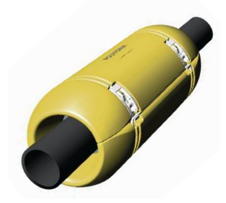
The POLYFORM® Sub FlowSafe is made from a rotomolded PE outer shell and filled with polyurethane (PUR) foam, guaranteeing a compressive strength of 500 mH20.
