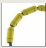
The Sub Flowsafe is made from a rotomolded PE outer shell and filled with polyurethane (PUR) foam, quaranteeing a compressive strength of 500 mH20
