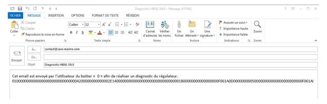
This information allows Save Marine technicians to make an accurate and distant diagnosis of the turbine and the electronic box which are the two most difficult components to monitor.
