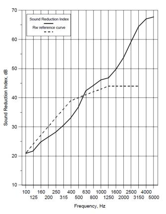
\*Mounted on 17mm composite bulkhead
