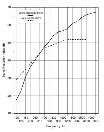
\*Mounted on 17mm composite bulkhead
