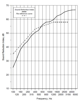
\*Mounted on 17mm composite bulkhead
