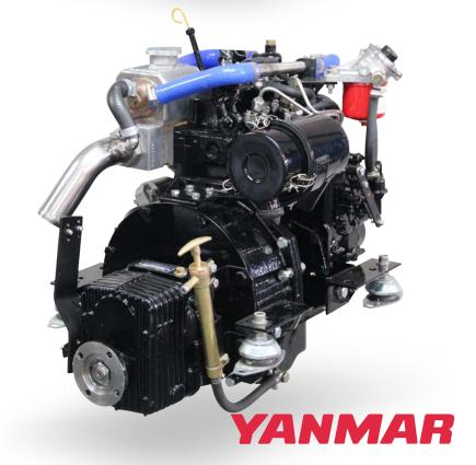
Naturally aspirated, 4 cylinder, 4 cycle in-line water-cooled diesel 270 kg dry weight Full size replaceable air filter for maximum filtration and noise reduction 50 amp 12V alternator
