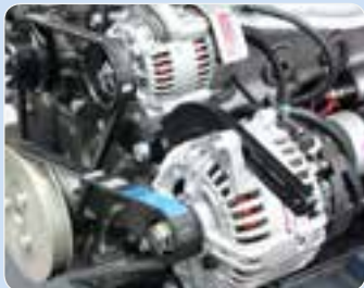
12 volt 50 amp and 140 amp alternators Fuel filter with water drain separator PRM 150 Hydraulic Gearbox
