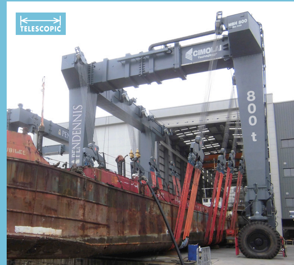
Capacity: 800 t - UK - Hydraulically adjustable track
