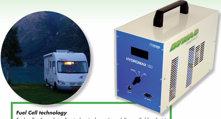
Fuel cells, through a direct chemical reaction, deliver reliable electrical energy, safely, quietly and without excessive generation of heat. When a vehicle's battery discharges to a certain point, the fuel cell automatically turns on and charges the battery. When the battery is sufficiently charged, the fuel cell turns off again. The system operates automatically and is therefore also ideal for use in remote locations, for security installations for example.
