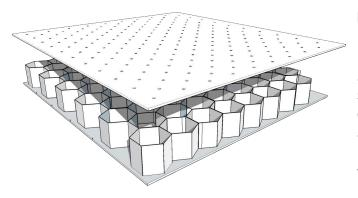
Luxboard A-QA is an innovative and refined product made of highest quality of materials and the latest manufacturing processes. Thanks to the "Helmholtz Resonance", the panels can be considered as reactive silencers with impressive low frequency absorption coefficients. Such results were previously only achievable by use of bulky & havyweight combinations. Luxboard A-QA is made of marine grade aluminium which is completely fibre-free, corrosion resistant, lightweight and robust.
