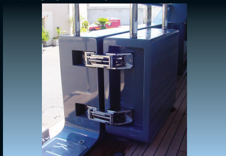
180° opening bulwark door hinge
