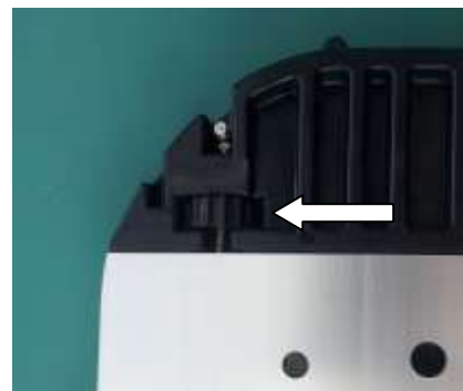
Thumb nut adjuster on rudder head for boat trim
