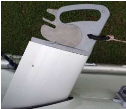
Safety clip attached to the shock cord
