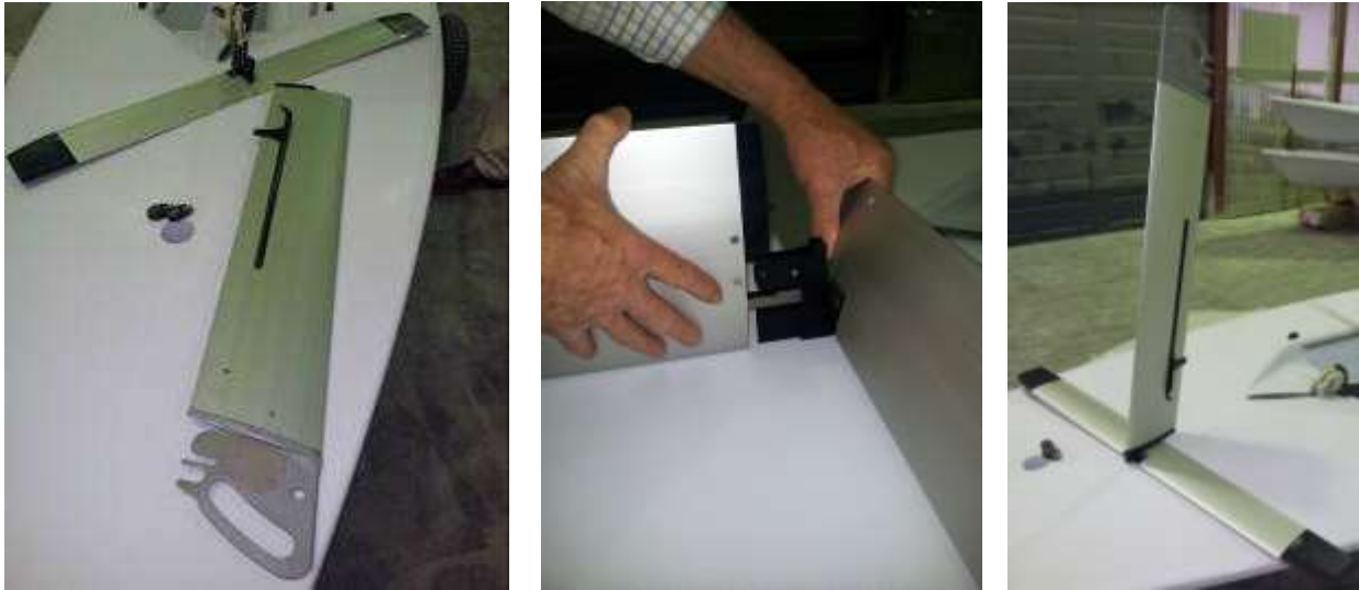
Assembly of Centreboard foil and lifting foil.
