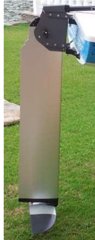
Rudder assembly including vertical rudder blade, horizontal foil and rudder box
