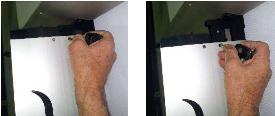
Depress the spring clip and pull the foils apart.
