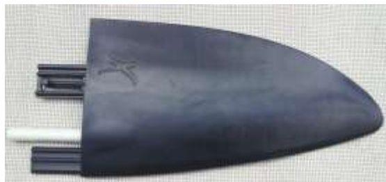
High lift Spitfire wingtip for light winds
