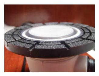
The purpose of the plastic disc is to ensure you have a solid contact to the hull of the boat. Later in this guide you will be applying epoxy resin to the boats hull and this plastic disc will protect the transducer face from the epoxy resin.
