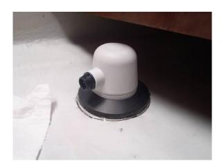
Example of a transducer that has been left in place to cure. This is how your transducer should look before you move to the next transducer.
