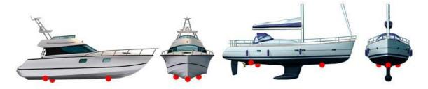
The transducers should be located towards the stern between the propeller and the rudder. One should be placed to port and the other to starboard approximately 30cm from the centre line.
