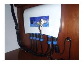
The unit above was installed in the aft port cabin on the outside of a locker, this gave good access to the main control panel, battery and also the Aft transducers
