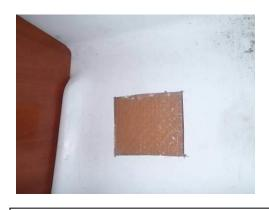
This area had a false floor in the starboard aft cabin and so required cutting to access the GRP hull. We used a Fein Multimaster tool with the saw attachment that was ideal.
