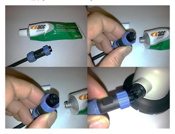
Apply only a small amount of silicon grease (approx. ½ pea or 0.5g) to the plug, ensure the grease is evenly spread over the connection. Then connect plug to socket.
