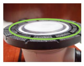
Apply epoxy to the ring area only (highlighted Green), avoiding contact with the plastic covering (highlighted red below)
