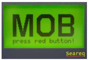
4. MOBOS<sup>®</sup>-Receiver has received an alert and shows MOB on its screen. Parallel a loud signal is audible.
