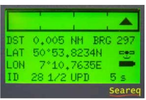
6. Just a short time later MOBOS<sup>®</sup>-Beacon has evaluated its valid GPS data which are instantly and automatically relayed to the MOBOS<sup>®</sup>-Receiver.
