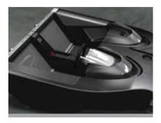
Future Fibres is leveraging the highest precision moulding technology the company uses to manufacture masts for the production of a roadster tube and main chassis. Designed by RPx engineers, this extremely light weight carbon fibre chassis offers excellent aerodynamics while remaining affordable.
