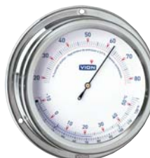
A130 CHR T + H • Curved, alcohol tube thermometer • Precision hygrometer with synthetic hair (+/- 2.5%)
