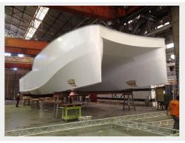
Along with the H2X engineers, the SAERTEX team tested and studied the potential use of SAERfix for this application. Right away, it became clear that these self-adhesive glass fibre reinforcements could be used by H2X to completely get rid of the spraying process.
