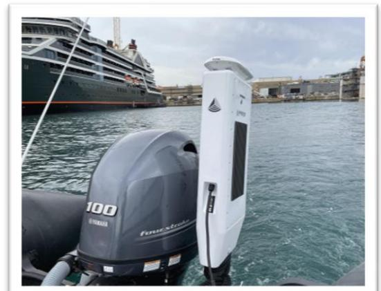
**WASSP W3 system configuration (Fixed Tender installation with fixed PC and video connection to MFD)**
