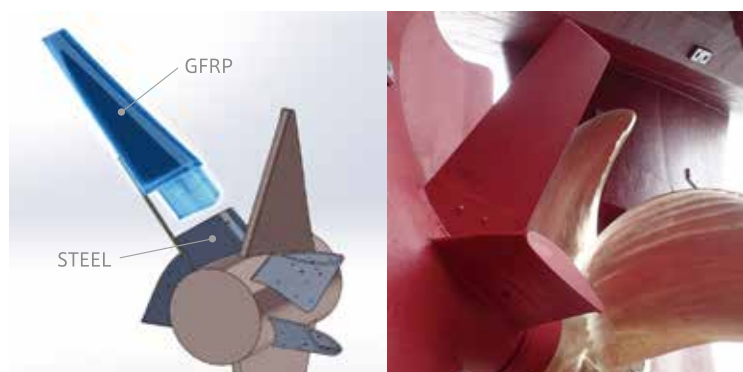
Fig.6 Construction and actual equipping of Composite Stator
