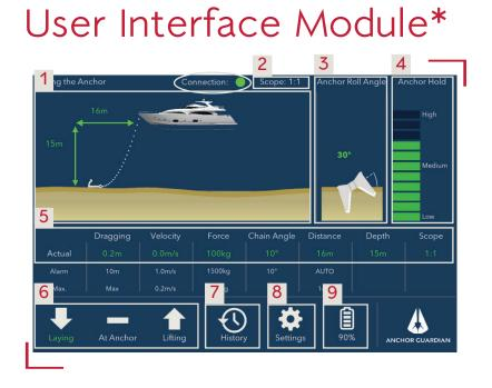
The user interface module translates information to the crew and communicates with the mother board for processing. It is the main point of interaction between man and machine.
