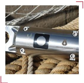
The anchor module is the heart and soul of AnchorGuardian and the eyes and ears of the captain and crew. Our proprietary movement detection technology allows the anchor module to detect sub-meter shifts and transmits this data in real-time to the user.
