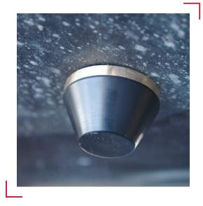
The boat module is the main communication hub that links users and modules of the AnchorGuardian solution. It consists of the hull mount boat transducer made of seawater resistant bronze alloy and the communication electronics integrated in a box. The boat module communicates underwater via ultrasound with the anchor module and above water via bluetooth or cable with the user interface.
