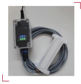
While the AnchorGuardian series product will use a patented wireless inductive solution to charge the battery of the anchor module, the prototypes still need manual attachment of a charging plate. This charging plate is equipped with a telescope handle and four alignment pins with magnets to align and fix the plate on the anchor module.
